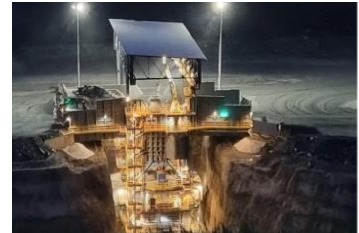
In-pit crusher at Sentinel
