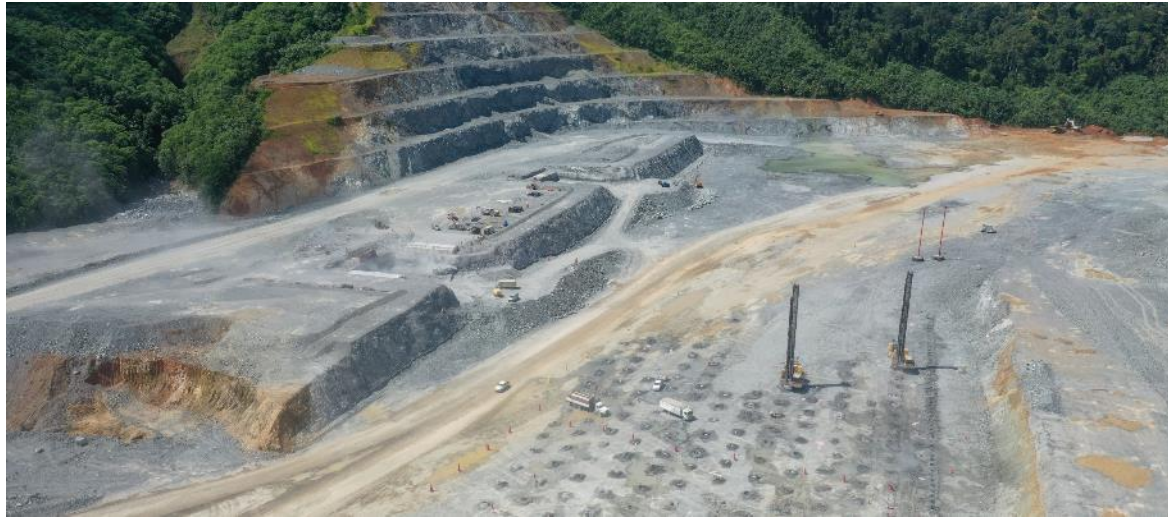
New Colina pit, drilling to blast for overland conveyor and access road to in-pit crusher
