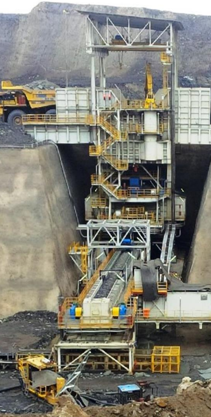
Semi-mobile in-pit crusher
