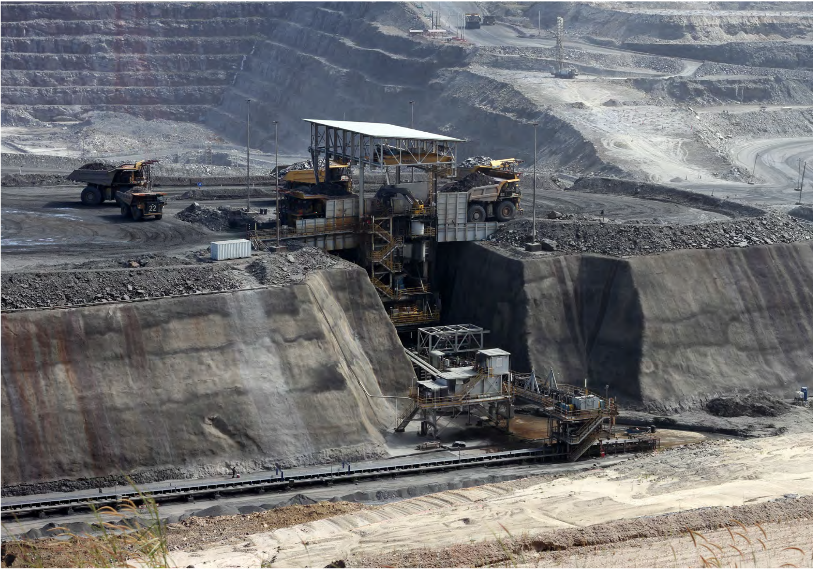
An in pit crusher and conveyor at the Company’s Sentinel mine, which contributed to GHG savings of almost 40,000 tonnes in 2020 through reduced use of the diesel-powered mining fleet.
