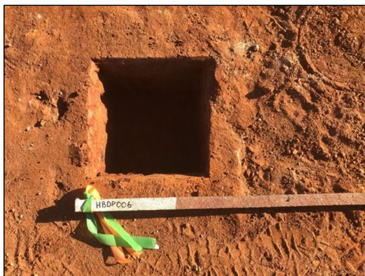
Figure 11-4 Density Sampling Pit (Hale-Bopp Mine) – (300 mm by 300 mm by 200 mm)
