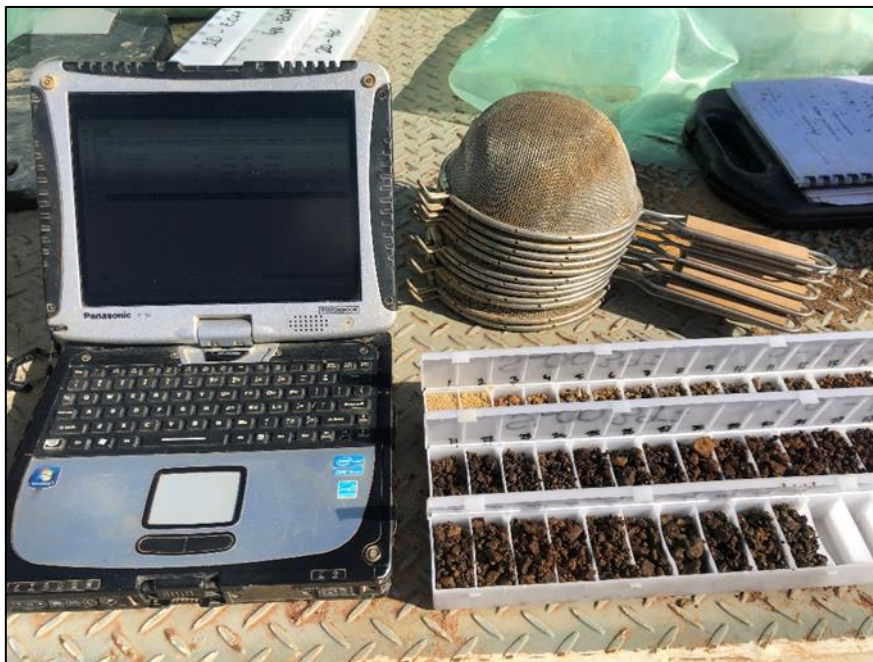
Figure 11-2 Ruggedised Laptop, Sieves and Logging Chip Trays for One Drillhole (2019)
