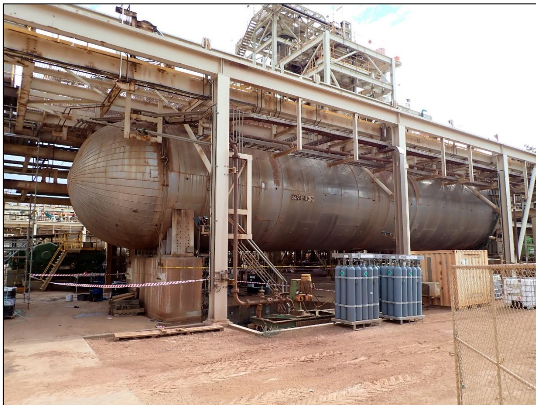
Figure 17-3 One of two autoclaves at RNO
