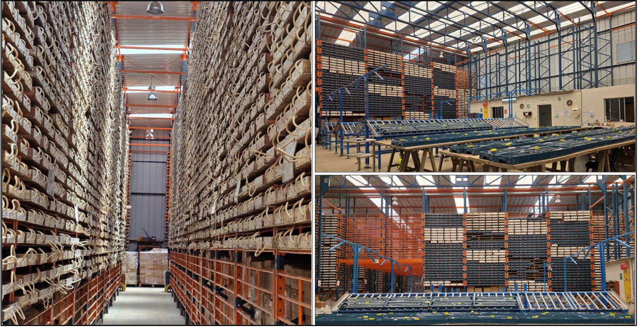
Figure 11-12 La Granja core shack showing logging tables and core storage racks. (source: FQM)
